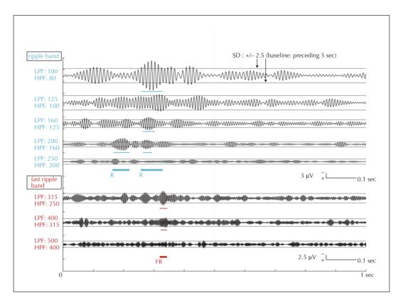
**Figure 2.** An example of the use of the automatic HFO detector. A wide band and eight subsequent narrow bands of the Finite Impulse Response (FIR) filter were applied. The ripple band consists of five bands (80-100, 100-125, 125-160, 160-200, 200-250 Hz) and the fast ripple band consists of three bands (250-315, 315-400, 400-500 Hz). Oscillatory activities larger than +/- 2.5 SD of the baseline and with four or more cycles of the central frequency band are detected as HFOs.
